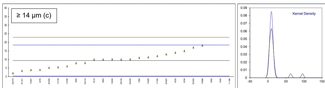
Determination of Level of Contamination acc. to ISO4406 scale on sample #22211; results in scale number
