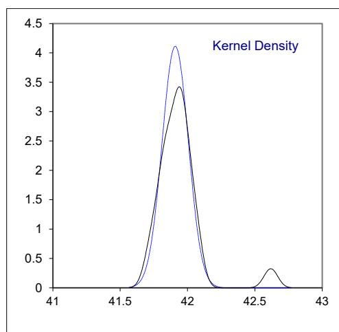
Determination of Kinematic Viscosity Stabinger at 100 °C on sample #22211; results in mm<sup>2</sup>/s
