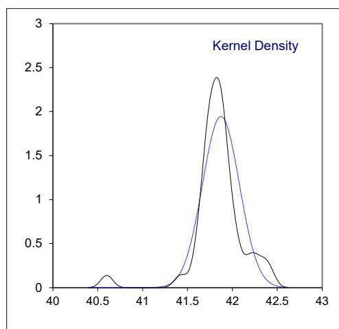
Determination of Kinematic Viscosity at 100 °C on sample #22211; results in mm<sup>2</sup>/s
